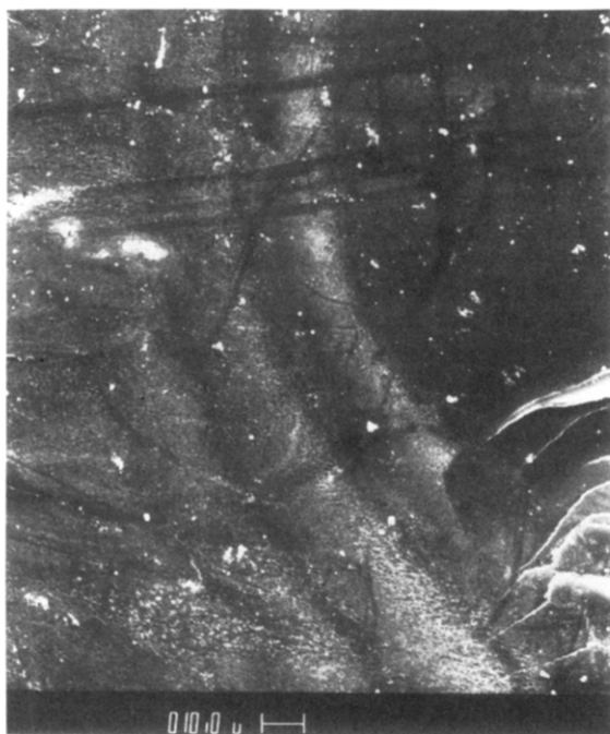
Figure 4. Portion of fatigue fracture surface of K salt ionomer with 4.1 mol % ion content tested at a stress amplitude of 11 MPa and at 5 Hz.
